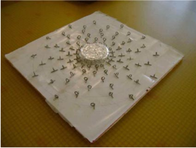
Figure 6. Experimental mock-up of a cloaking device based on canonical spirals [47].
