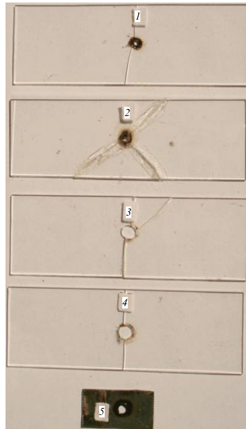
Figure 3. View of holes after penetration by ball lightning: 1 and 2 — holes 2 and 3 mm in diameter with melted edges in a glass plate 1 mm thick at a discharge current of 25 and 50 A, respectively; 3 — a smooth-edged hole more than 5 mm in diameter obtained after removal of the melted rim of holes 1 and 2 ; 4 — a hole produced in a glass plate without a wire but when the glass plate had a small hole (nearly 0.5 mm in diameter) before the discharge; 5 — a hole 4 mm in diameter in a 0.5-mm metal plate.
