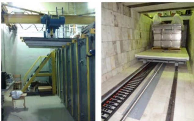
Figure 24. (Color online.) General views of the passive shielding on the inside and on the outside. The range of shifts of the detector within the neutrino channel amounts to 6–12 m from the reactor core.
