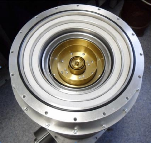
Figure 2. Triband feed in a cryostat (without a radio transparent window).
