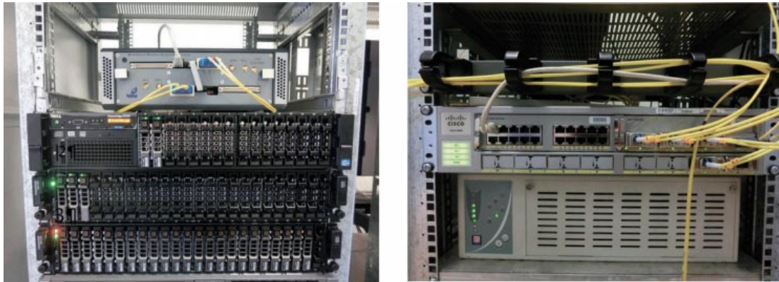
Figure 4. (a) Prototype of a data buffering and transfer system. (b) Double-channel broadband signal converter.
