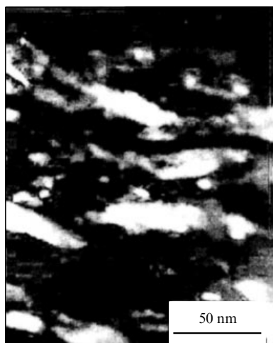
Figure 5. Nano-sized crystals of \alpha -martensite produced under cryogenic ( T = 77 K) deformation in Fe–Ni–Cr–Al alloy; dark-field electron microscopy image in \alpha -phase reflection.
