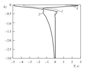
**Figure 8.** Examples of dimensionless profiles of temperature perturbations at the vertical line x = 0 for  $\chi \alpha \gamma_T / \kappa \beta \gamma_S = -1$ ,  $kh_T = 1$ , and  $kh_S = 0.05$  [39]. Curves I and 2 respectively pertain to one- and two-component media; curve 3 is the normalized profile of the vertical velocity w in the case of a two-component medium.
