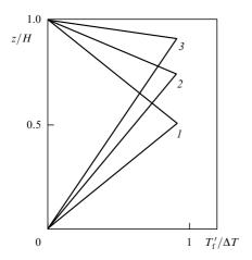
**Figure 4.** Deviations of temperature from the linear background distribution for various values of the parameter a and a piecewise linear dependence  $\tau(z_0)$  with  $\eta = 2$ :  $a \le 1$  (1), a = 0.5 (2), and a = 0.8 (3).
