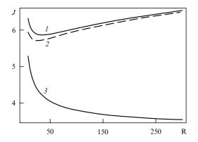
**Figure 11.** Neutral curves on the plane (R, J) for various boundary conditions and values of the parameter  $\xi$ . Curves I and 2:  $\xi = 80$ , 150 and  $b_T = b_S = 100$ ; curve 3:  $\xi = 80$ ,  $b_T = 100$ , and  $b_S = 0.015$ .
