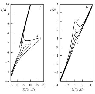
**Figure 5.** (a) Vertical distribution of temperature and (b) admixture concentration at the symmetry axis of the perturbation for  $\tau(z_0) = 1/(1+z_0^2)$ ,  $\eta=-5$ , and various values of the parameter a: a=0.4 (I), a=0.8 (2),  $a=a_{\rm cr}=8\sqrt{3}/9\approx 1.54$  (3), a=3 (4).
