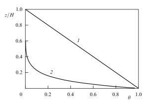
**Figure 13.** Example of the deformation of the background vertical temperature profile by descending fluid motions. Curve *I*: the vertical background motion is absent, curve 2: the profile for  $\varpi = H/h = 10$ .
