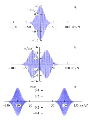
**Figure 1.** Horizontal distributions of buoyancy at the midlevel at successive time instants t = 0 (a), t = 20 (b), and t = 40 (c). The time scale is  $H/\pi c$ .
