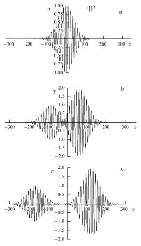
**Figure 14.** Temperature distribution (44) for time instants (a) t=0, (b) t=60, and (c) t=120. The values of x, t, and T are respectively normalized by  $L_{\rm R}$ ,  $L_{\rm R}$ / $\bar{U}$ , and  $\varepsilon_T$ .
