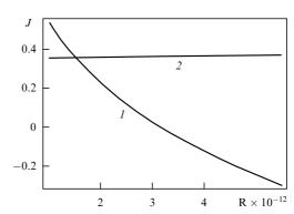
**Figure 12.** Neutral curves for large values of R,  $\xi = 80$ , and  $b_T = 100$  for  $b_S = 0$  (curve *I*) and  $b_S = 0.015$  (curve *2*); curve *2* is normalized by 10.
