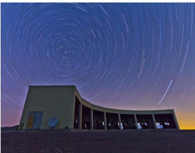
Figure 4. Middle Drum station comprising 14 telescopes recording fluorescent emission of the atmosphere. The long-exposure night shot was contributed by B Stokes.
