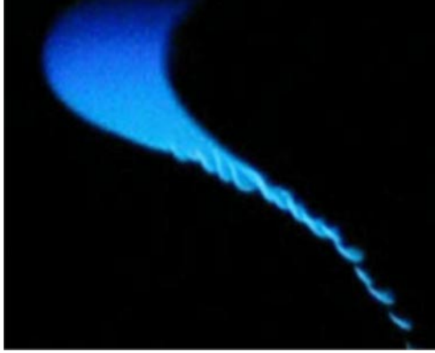
Figure 3. Screw structure of a whisker being drawn out of a spin nucleus.
