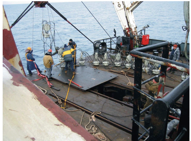
Figure 2. Deployment of a 16-element transmitting complex to its underwater position from the deck of the research vessel.
