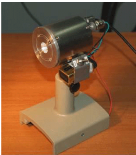
Figure 5. Pyroelectric terahertz pulse energy meter.
