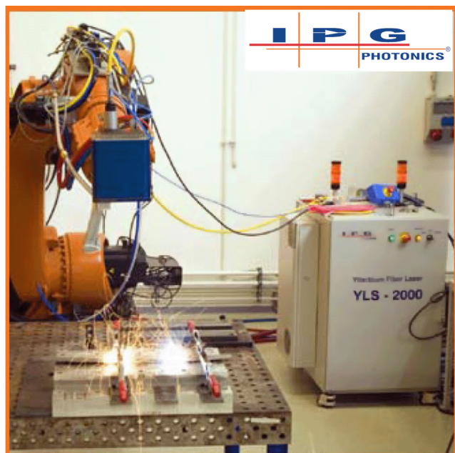
Figure 8. Laser technology system using a high-power fiber-optic laser from IPG Photonics ( www.ipg-photonics.com ).
