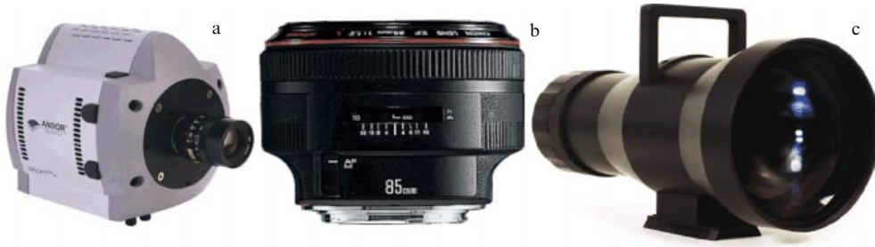
Figure 10. Possible mass-produced components of the projected system: (a) Electron-multiplying Andor iXon EM +888 CCD matrix with 1024 \times 1024 pixels, each 13 \mu\text{m} in size; (b) Canon EF 85 f/1.2 L USM II objective capable of imaging a 9 \times 9 degree field onto this matrix for a scale of 31''/\text{pixel} ; (c) Marshall Electronics 140 mm f/1.0 objective, which affords a 5.4 \times 5.4 degree field for a scale of 19''/\text{pixel} .
