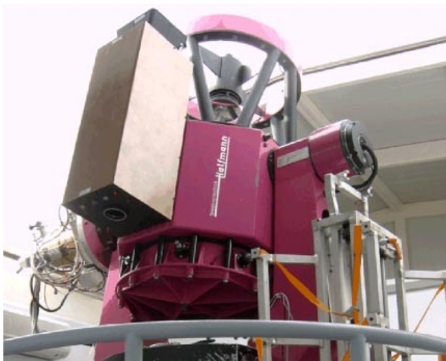
Figure 2. Image of the TORTORA camera mounted on the REM robotic telescope in the La Silla Observatory (ESO, Chile).
