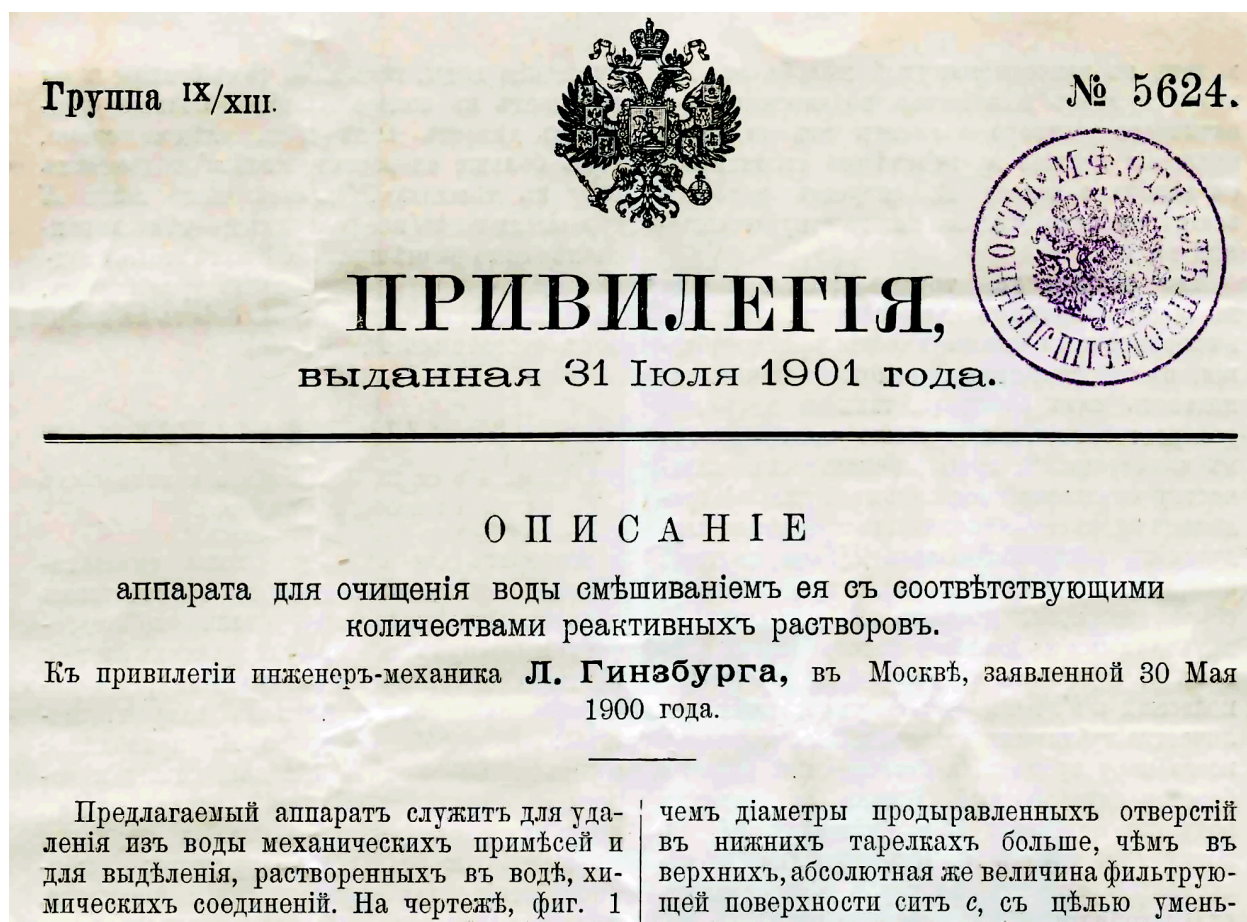
Photo 6. A portion of the first page of the patent (known at the time as a 'privilege') of mechanical engineer Lazar Efimovich Ginzburg for an apparatus for water purification (application submitted on 30 May 1900).
