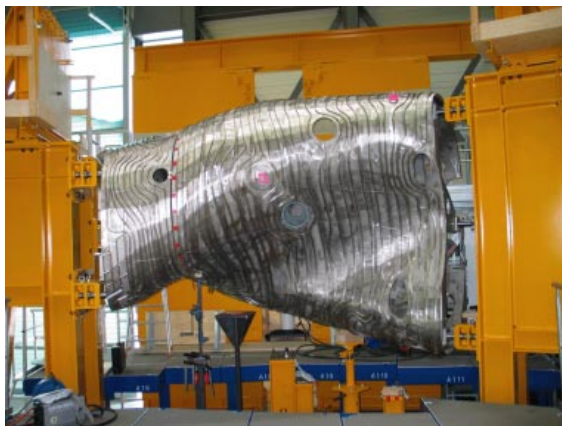
Figure 9. A fragment of the W-7X vacuum chamber (half the module).
