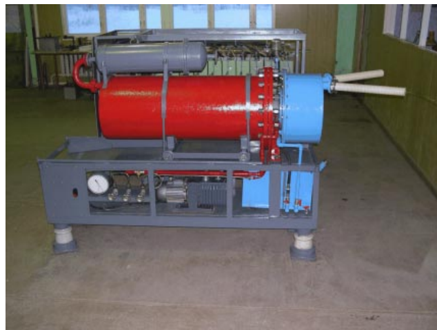
Figure 11. Mobile explosive simulator of lightning strokes based on a magnetic explosion generator.
