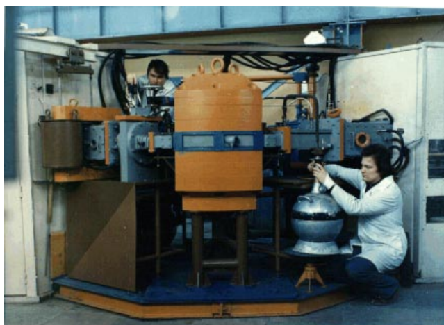
Figure 7. Ion-beam accelerator ILU. Ion energy: up to 40 keV; total current: up to 30 mA; magnetic field: up to 5500 Oe; processed area: 15 \times 20 \text{ cm}^2 ; ion species: throughout the Periodic Table.
