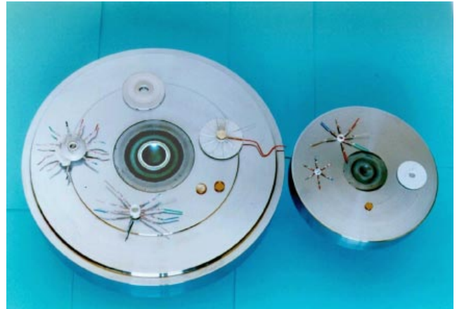
Figure 8. High-pressure cells of the toroid type.
