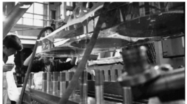
Hydrogen bubble chamber of size 2 m on the assembly bench.
