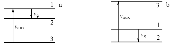
Figure 1. Schematic of the population inversion using auxiliary radiation (pumping). \nu_{\text{aux}} , auxiliary radiation frequency; \nu_g , signal frequency that provides generation.
