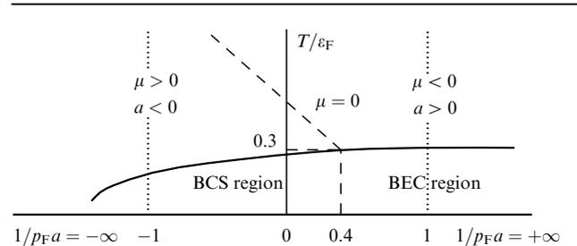
**Figure 5.** Phase diagram of a resonant Fermi gas in the 3D case. Regions labelled BCS and BEC correspond to Cooper pairing and to Bose condensation of local pairs, respectively.
