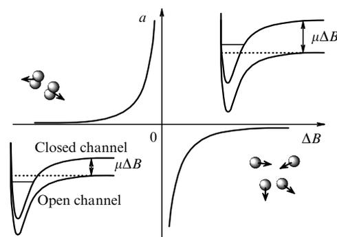
**Figure 1.** Schematic illustration of the Feshbach effect. Applying a magnetic field causes two energy terms to cross in the open and closed channels, changing the system from one with a bound state for  $a > 0$  to one with a virtual state for  $a < 0$ .  $\Delta B = B - B_0$  is the deviation of the magnetic field  $B$  from the Feshbach resonance field  $B_0$ , and  $\mu$  is the magnetic moment of the atom.
