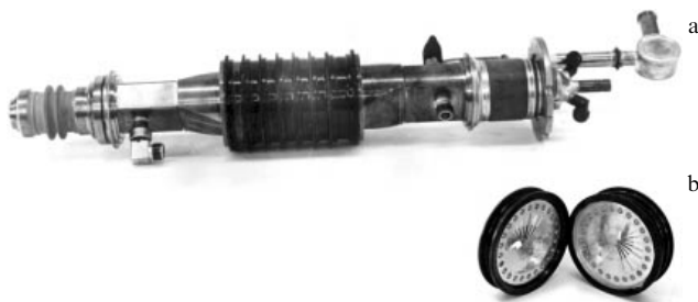
Figure 17. Experimental variant of a CPTWT (a) and fragments of the slow-wave system in the form of a spatially twisted two-row comb (b).
