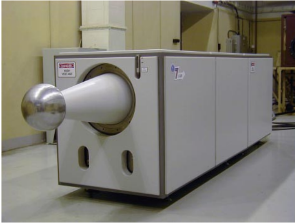
Figure 9. S-5N generator. The output voltage is 400–1000 kV, the current through the load is 1–3 kA, and the pulse duration (FWHM) is 30–50 ns. Pulse repetition rate: 300 Hz (constantly), 900 Hz (a 30-s long pulse packet). Average input power: 18 kW (constantly), 45 kW (a 30-s long pulse packet). Overall dimensions of the body: 3.5 \times 1.4 \times 1.1 m; mass: \sim 2800 kg.
