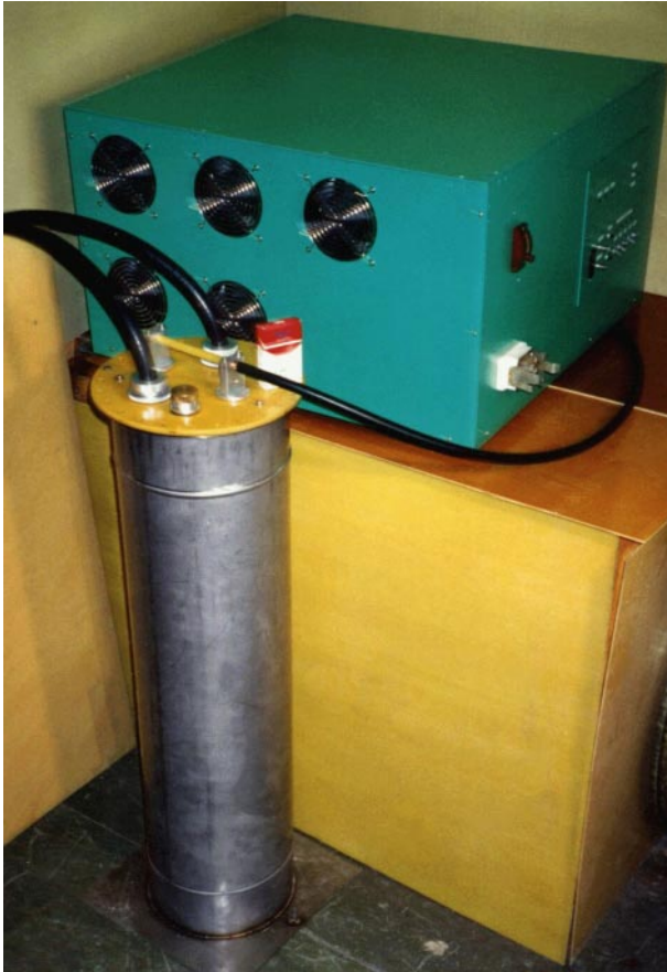
Figure 6. Generator of high-power nanosecond pulses. The pulsed voltage is 70 kV, the pulse current 3 kA, the rise time 3–5 ns, the pulse energy 2 J, and the repetition rate may be as high as 2 kHz.
