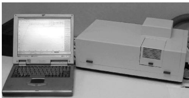
Figure 2. Portable CDS-2 dichrometer for high-sensitivity measurements within an extended spectral range (200–750 nm).
