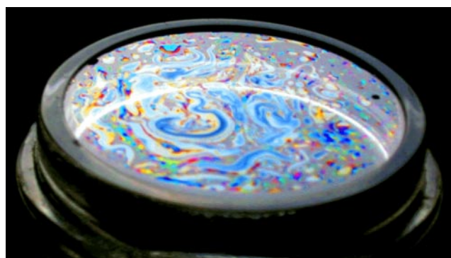
Figure 15. Rigid, dry, and transparent soap film with the diameter 65 mm manifesting a fixed interference pattern in reflected light.
