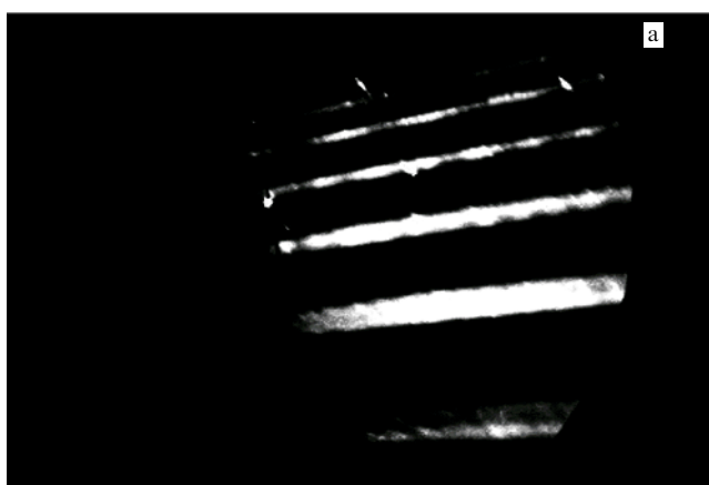
Figure 13. Laser tracks on a concave soap film. The tracks are distorted at the inhomogeneities formed by large dust particles.
