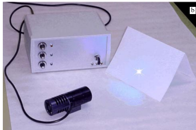
Figure 3. (a, b) Photos of single-frequency lasers radiating in the blue spectral domain.
