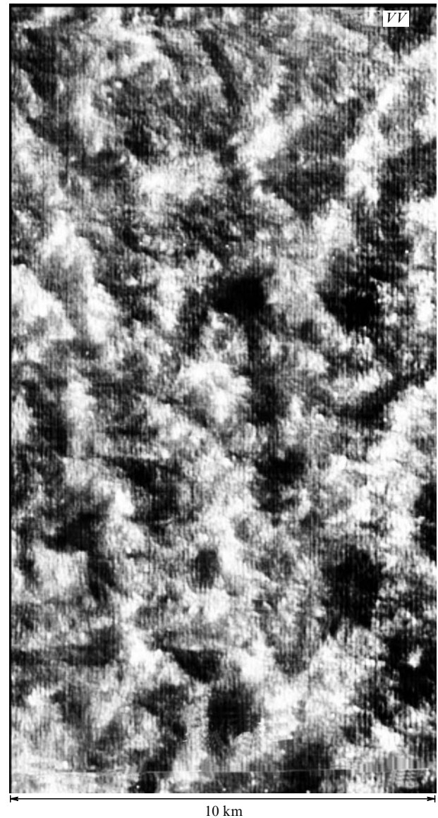
Figure 9. Sea-surface radar image obtained with a vertically polarized signal and showing convective cells, offshore from Kamchatka, 28 August 1985. Wind velocity was 6 \text{ m s}^{-1} ; T_{\text{air}} - T_{\text{water}} = -6.5^\circ\text{C} .
