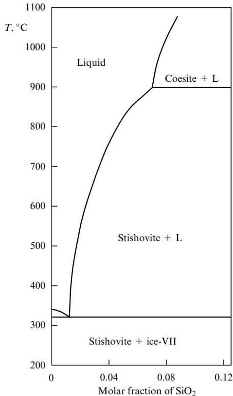
**Figure 2.** Part of the  $(T, x)$  phase diagram of the  $\text{SiO}_2\text{-H}_2\text{O}$  system at 9 GPa.
