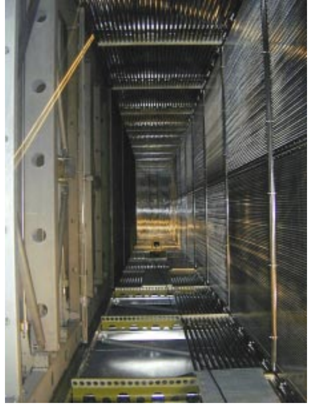
Figure 20. Inside the 300 t ICARUS sub-module, a view of one of the two mirror drift volumes. The presence of the wire chambers on the left can be inferred from the oblique pattern on the left due to the reflection of light.
