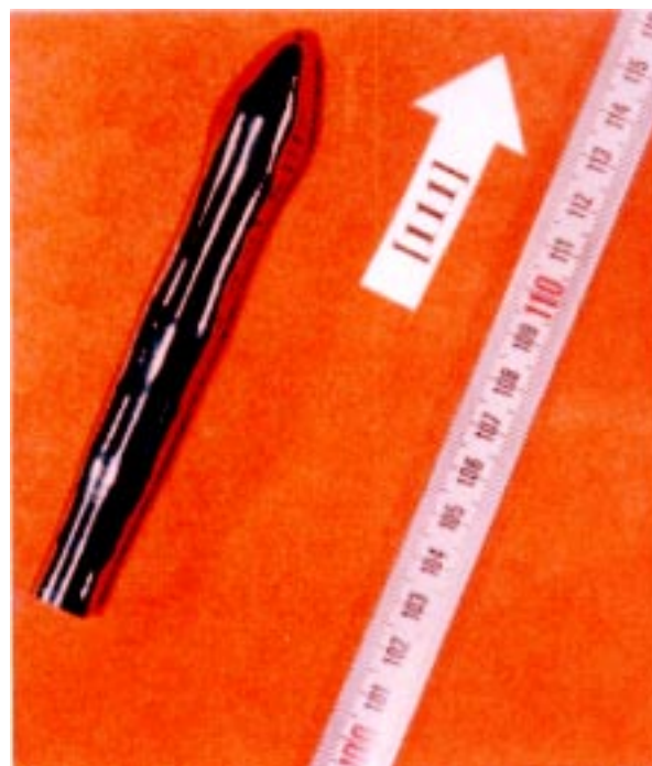
Figure 2. Single crystal of an isotopically pure (99.99%) germanium isotope ^{70}\text{Ge} .
