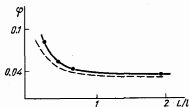
FIG. 7. Theoretical (broken line) and experimental (solid line) dependences of \varphi_i on L/l for molecules of PBA.
