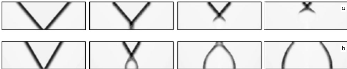
Figure 18. Interaction of two plane U-waves at different angles \alpha between the fronts ( L_x \times L_y = 150 \times 50 , \Delta t = 20 ) [71]: (a) \alpha = 80^\circ , (b) \alpha = 60^\circ .
